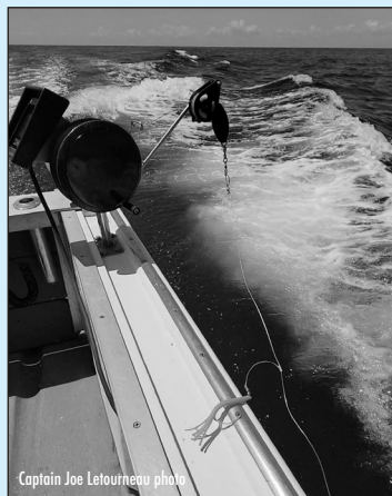
DNG automatic jigging machine at sea.
