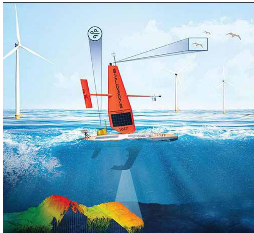
Example of saildrone technology, including multibeam bathymetry to map the ocean bottom, 24/7 autonomous operations monitoring with real-time data transmission via satellite communications, and wind powered for propulsion. Credit: Saildrone.
