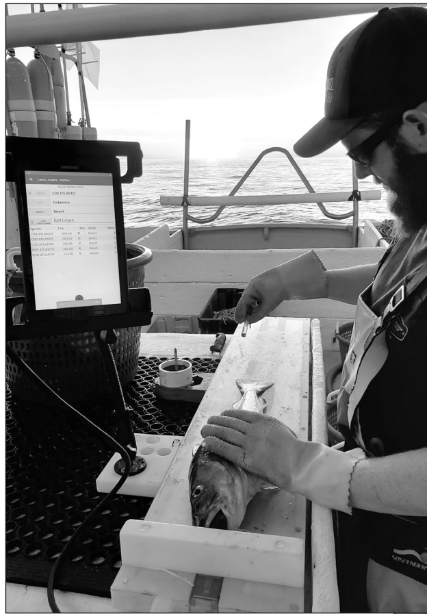
CRB staff member Jack Wilson measuring an Atlantic cod using a digital fishboard and new tablet application during the fall 2020 bottom longline survey.
